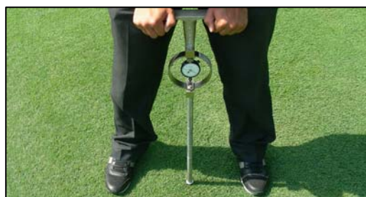
Figure 4. Head of penetrometer is forced into soil surface.
