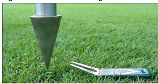
Figure 3. Conical head of the soil penetrometer.
